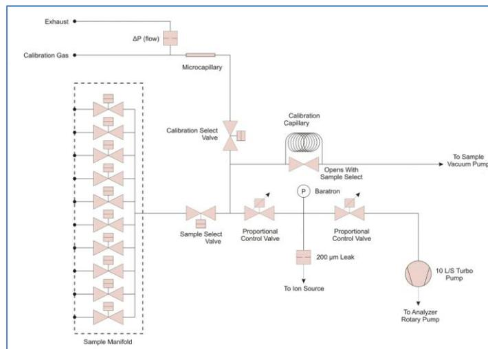
Figure 4: Prima PRO 's variable pressure inlet
