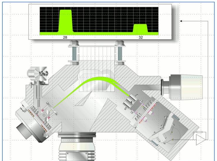
Figure 3: Prima PRO's magnetic sector analyzer
