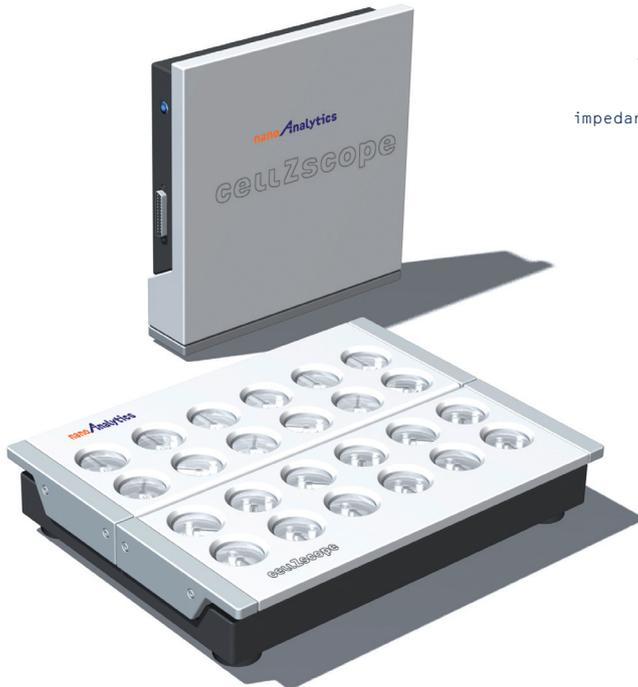
The cellZscope is a new device for measuring the transepithelial or transendothelial electrical impedance of cell layers under physiological conditions. It is computer-controlled and allows automated, long-term monitoring experiments with up to 24 different cell cultures simultaneously.
