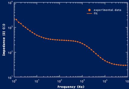
Typical frequency-dependence of the electrical impedance ( $Z$ ) of an epithelial or endothelial cell layer: the fit curve is based on equivalent circuit modeling. The cellZscope software performs full automatic data analysis and provides the user with cell-related parameters such as the transepithelial electrical resistance (TER) and capacitance ( $C_{cl}$ ).
