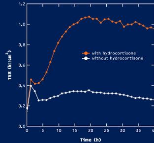
Time-resolved monitoring of the transepithelial electrical resistance (TER) of primary cultured endothelial cells derived from porcine brain microvessels, incubated in serum-free medium supplemented with hydrocortisone (orange curve) and without hydrocortisone (white curve): the experimental data reveal that the TER of the confluent cell layer increases with time in the presence of hydrocortisone. This effect is attributed to a pronounced barrier strengthening of the cerebral endothelial cells.
